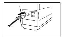
Insert the AC adapter's power plug to an AC outlet (100-240 VAC, 50-60 Hz).
